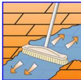
△ Important Advice: only in case of very stubborn residues or efflorescence should Lithofin MN Builders' Clean be used. The tiles are not resistant to acid, and their appearance will be altered by acidic cleaners. Dilute product heavily (approx.
