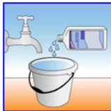
All cement residues must be removed from the surface. Use Lithofin MN Power-Clean diluted with water 1:10 to achieve a clean surface. A polishing machine with a white nylon pad will help cleaning the surface quickly and efficiently.
